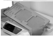
Hold the **Deck** (6) with both hands and place it over the corresponding positioning studs. Press down firmly until you hear a click.
